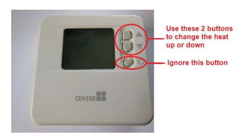
NOTE: "The Display" above shows the room temperature. After you change the heat, "The Display" goes back to showing the room temperature.
